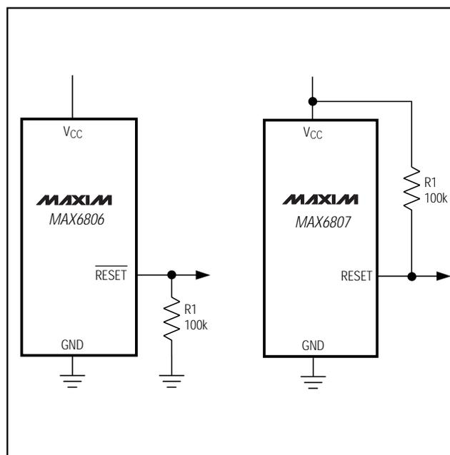
Figure 4.  $\overline{\text{RESET}}$  / RESET Valid to VCC = Ground Circuit
