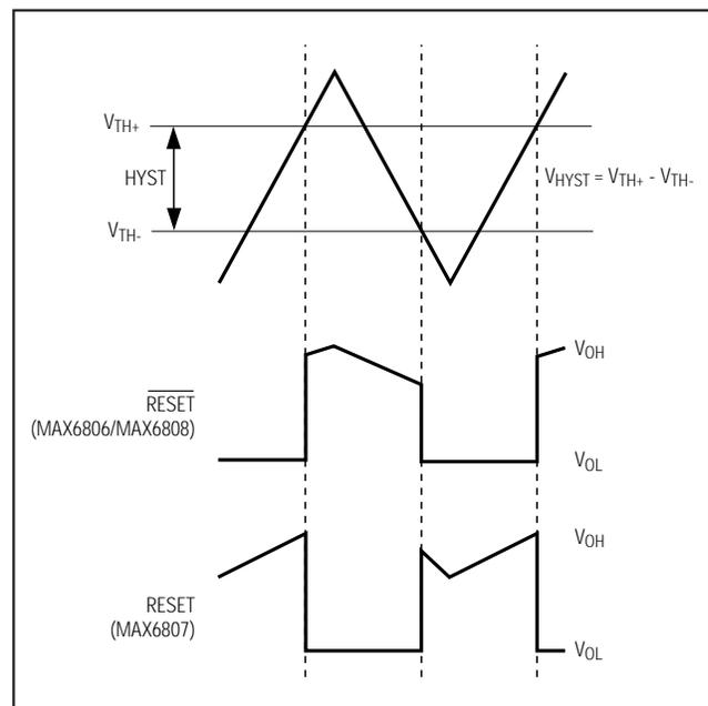
Figure 2. Input and Output Waveforms with  $V_{\text{CC}}$  Varied
